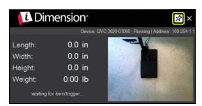
Dimensions are updated in the wedge application window each time the dimensioner is triggered. The image window shows the dimensioned item until it is removed.
