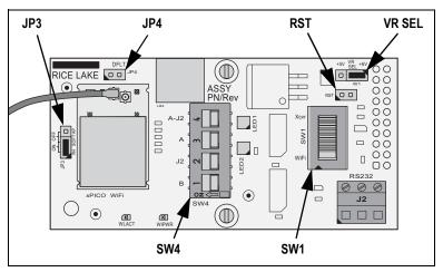
Figure 2. Jumper and Switch Locations on the WLAN Option Board
