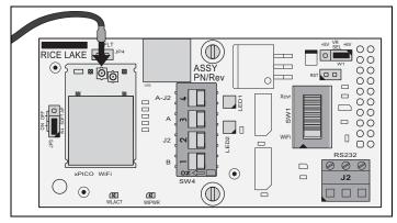
Figure 3. Antenna Connection Location
