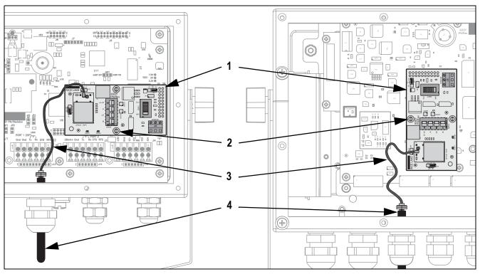
Figure 1. WLAN Option Parts Breakdown (Inside CW-90 [left] and 720i [right])
