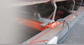
Belt scale model 311M is suitable for most belt widths, applications and constructions (with both idler stations and flat rollers).
