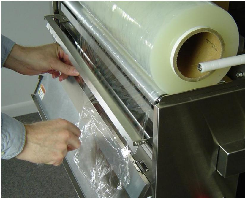
Figure 6.1.5. Tear the Film Straight
