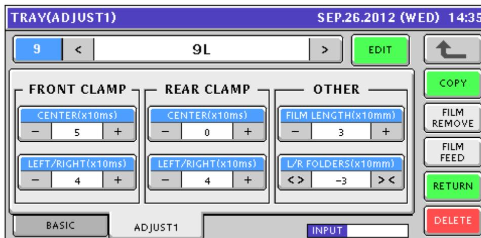
Figure 7.4.2. Tray Wrapping Adjust Settings
