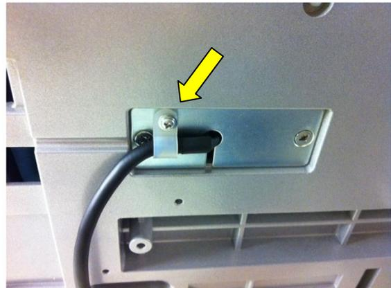
Figure 3.4. Wrapper to Scale Communication Cable Connection
