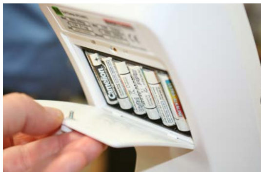
Figure 2-4. Batteries in Battery Chamber
