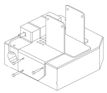
Figure 3-10. Reinstall Scanning Head Mounting Screws
