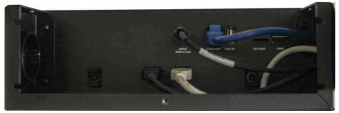
Figure 3-5. Scanning Head Connections
