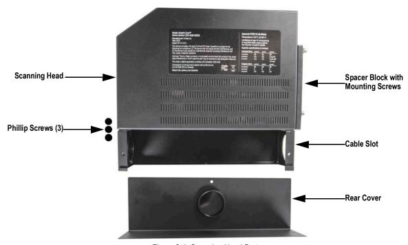
Figure 3-1. Scanning Head Parts
