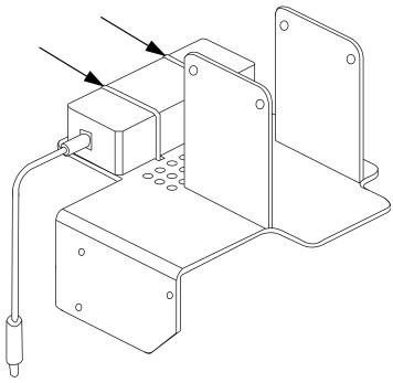
Figure 3-7. Secure Power Supply
