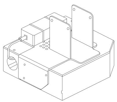
Figure 3-8. Mount the Bracket to Scanning Head
