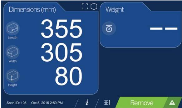
Figure 2-1. Operator Touchscreen Display
