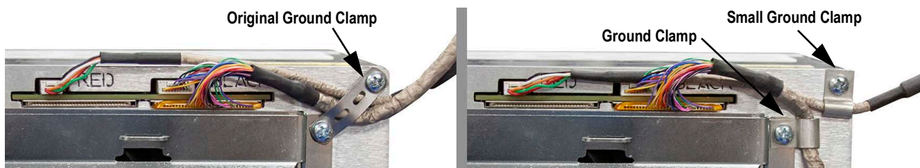
Figure 2-19. Controller Box Shield Grounding
