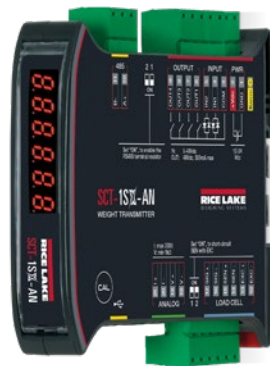
Removable Terminal Blocks Simplify Wiring
