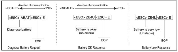
Figure 5-2. Diagnose Battery Examples
