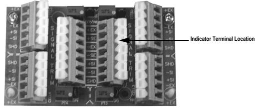
Figure 2-2. Junction Box Wiring
