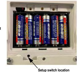
Remove four screws to access setup switch
