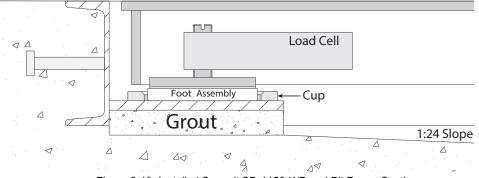
Figure 2-10. Installed Summit SD-1150-WP and Pit Frame Section
