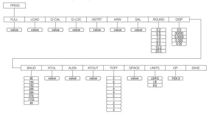
Figure 4-3. Programming Mode Menu Structure
