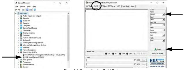
Figure 5-4. Connecting to a Serial Port
