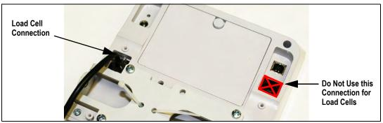
Figure 2-8. Load Cell Connection Point
