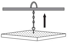
Small Platform (5 ft x 5 ft or smaller and/or 10,000 lb or less capacity) Use one 1/2 in eye bolt, insert into threaded hole in center of top plate for lifting.
