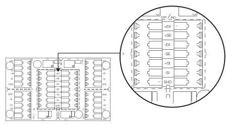
Figure 2-3. Expansion Port Wiring Location
