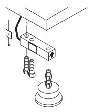
Figure 4-1. Load Cell Assembly
