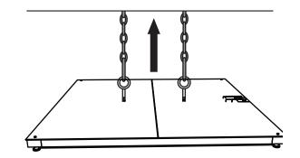
Large Platform (Larger then 5 ft x 5 ft, and /or more than 10,000 lb capacity) Use two 3/4 in eye bolts, insert into threaded holes in opposite corners of top plate for lifting.
