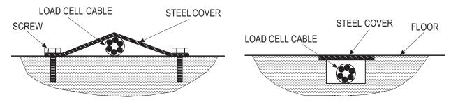
Figure 2-5. Cable Routing
