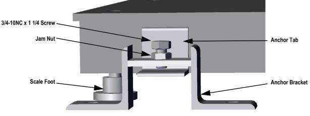
Figure 2-2. Anchor Bracket Installation
