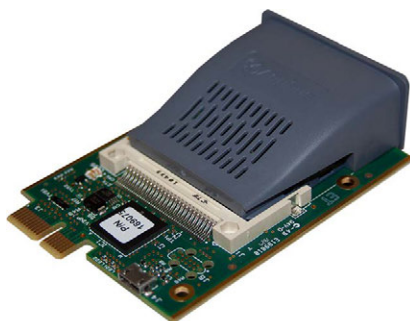
Carrier Board with Module
