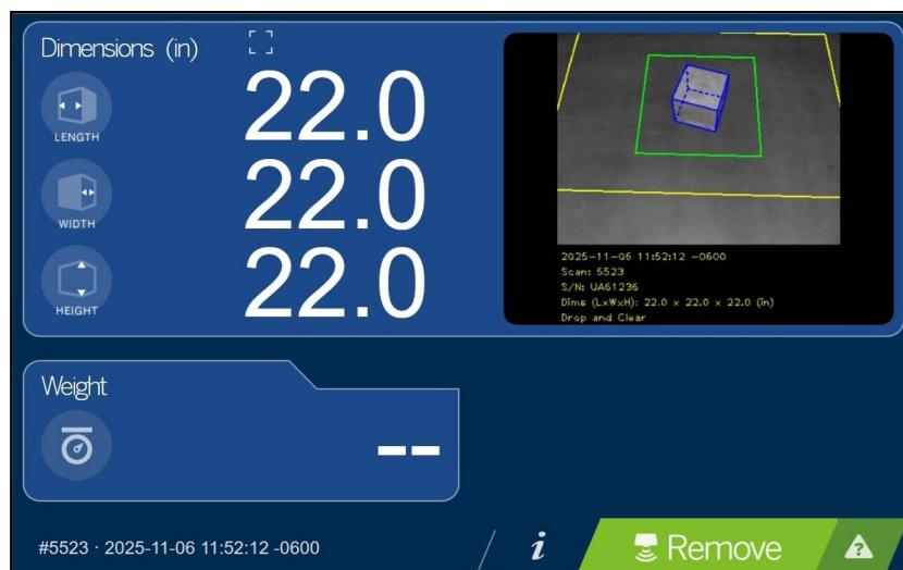
Figure 6-43. Hanging Dimensioner Calibration Verified
