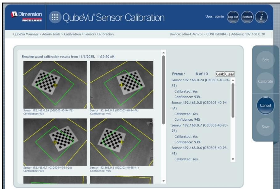
Figure 6-22. Calibration Object Under Dimensioner
