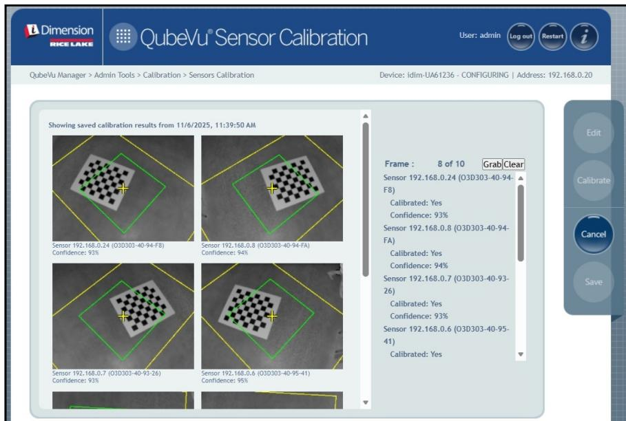
Figure 6-22. Calibration Object Under Dimensioner
