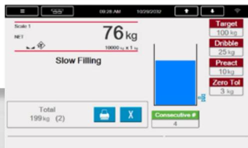
For repetitively filling one ingredient to a specified weight value.
