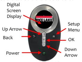
Figure 3-1. Handheld Controller Key Functions
