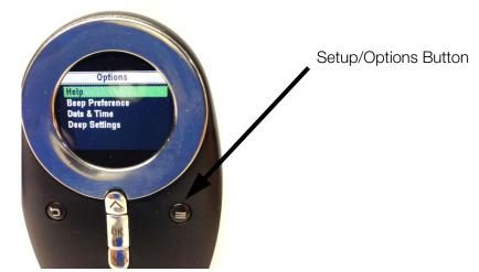
Figure 4-3. Setup/Options Button Location
