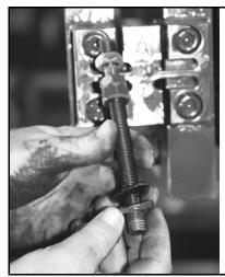
Ensure flexure rod threads are free of debris and paint by running a nut the full distance of the rod.
