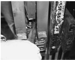
Figure 3-20. Center Load Cell
