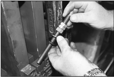
Figure 3-18. Install Spherical Washer Set
