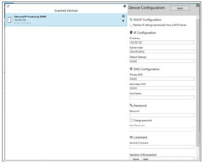
Figure 3-3. IP Configuration Utility - Enter Network Settings
