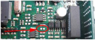
Figure 2-11. Soldered Jumper
