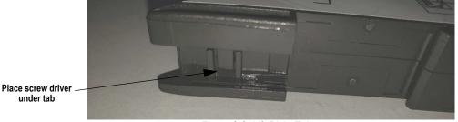
Figure 2-3. Lift Right Tab
