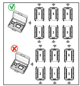
Figure 2. Wheel Weigh Pad Positioning
