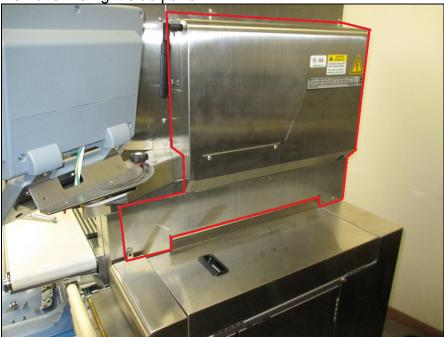
Step #3-Remove the three bolts shown in the picture below
