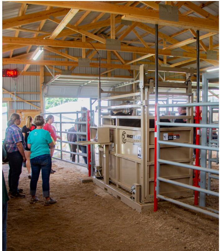
Choosing a Legal for Trade scale is step one of this new regulation. Step two is maintaining that scale to ensure its accuracy. It is necessary to work with a state-licensed scale service company to ensure the scale is in proper operating condition for fair market pricing based on animal weight. Most Legal for Trade scales must be calibrated at least once every year, but the Weights and Measures departments of different regions may require more frequent calibrations.
