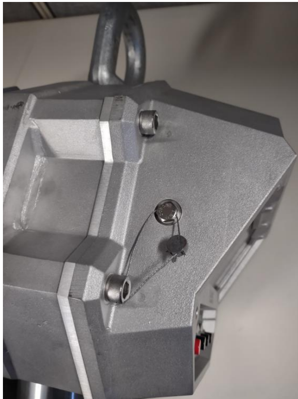
Typical Sealing / Scellage typique
