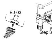
Connector inside the option slot
