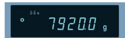
**Overall Capacity Indication** is a unique and helpful feature. By indicating how much of the balance's capacity has been filled, the risk of overloading the balance is minimized.
