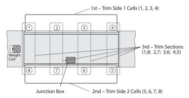
Figure 7-1. Load Cell Trimming Diagram
