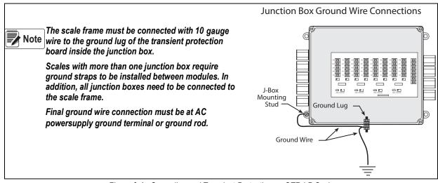
Figure 6-4. Grounding and Transient Protection on OTR-LP Scale
