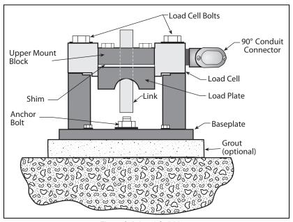
Figure 8-1. Load Cell Mount
