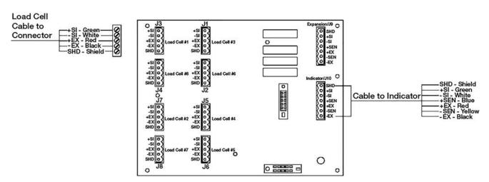
Figure 5-1. Junction Box Wiring and Conduit Runs for a Four Section/Three Module Scale
