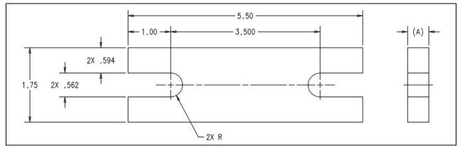
Figure 4-5. Example Shim Dimensions
