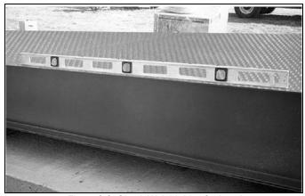
Figure 3-8. Check Weighbridge for Level
