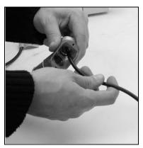
Figure 4-2. Insert Load Cell Cable Through 90° Fitting
