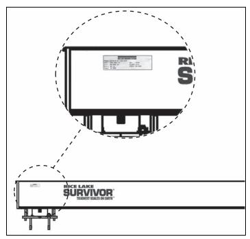
Figure 7-7. Serial Tag Placement
