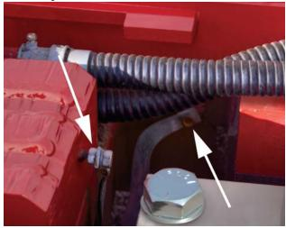
Figure 6-2. Inter-Module Ground Strap
