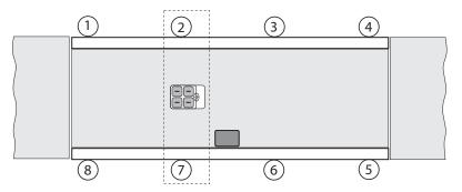
Figure 7-5. Trimming Paired Sections 2:7, 3:6 and 4:5
