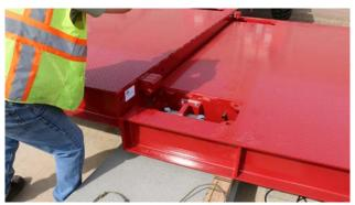
Figure 3-6. Pin and Receptacle Interface
