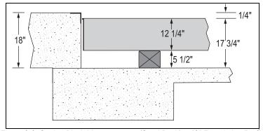
Figure 2-2. Setting Block Measurements (Steel Deck) – 18" Foundation Profile
