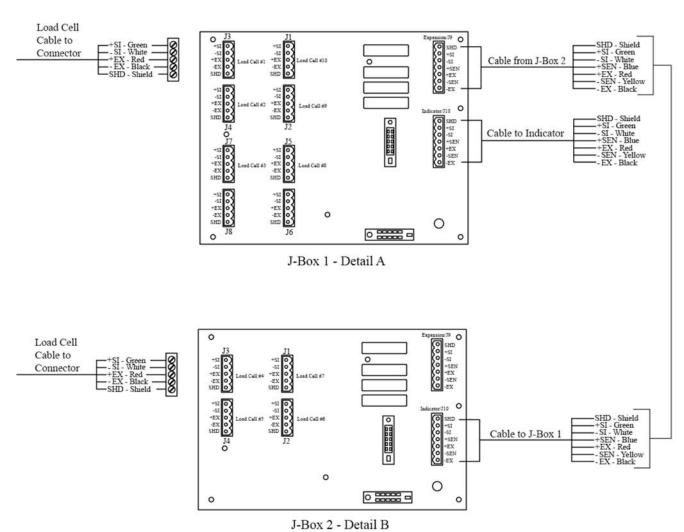
Figure 5-2. Junction Box Wiring and Conduit Runs for a Five Section/Four Module Scale
