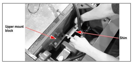
Figure 4-6. Shim Installation (Option 1)
