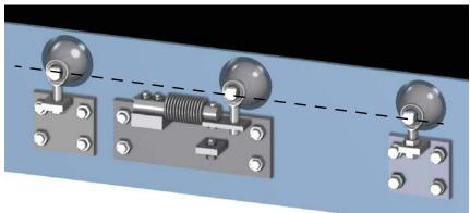
Figure 2-8. Install Side Bracket on Trailing Idler
