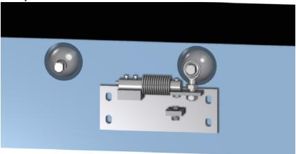
Figure 2-1. Align Rod with Idler
