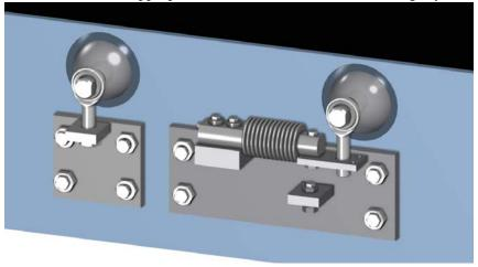
Figure 2-7. Secure Side Bracket
