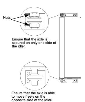
Figure 2-4. Secure Axle on Only One Side of Idler
