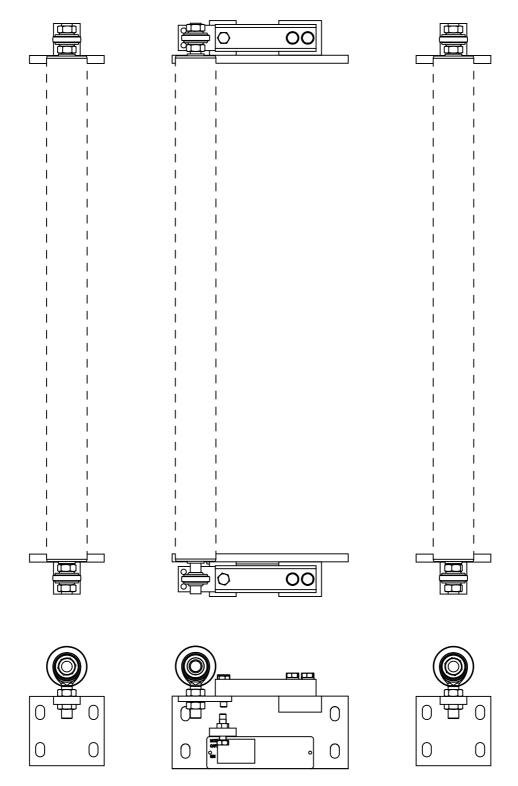
Figure 3-4. MASTER Series 421 Belt Scale Layout
