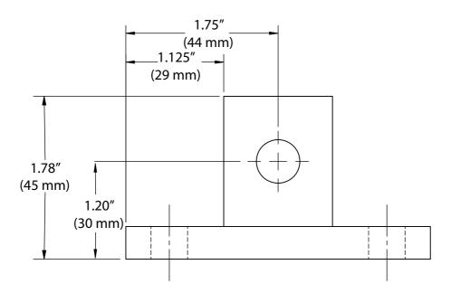
Figure 3-3. Side Bracket Dimensions
