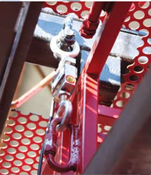
Left: Jason McDonald, Master Scales. Above: Five hundred pound S-beam load cells are used in the weigh basket. The picker can hold 1700 to 2000 pounds of cotton or 350 test plots before it dumps the load into boll buggies.
