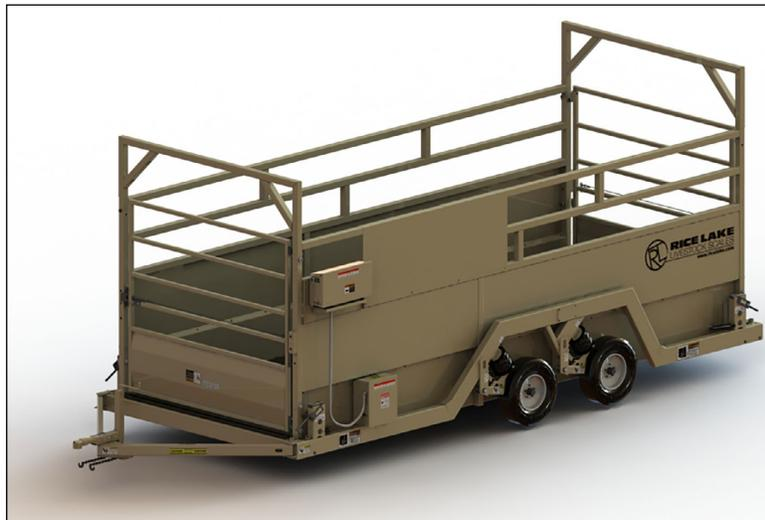
Figure 1-1. MAS-M Mobile Group Livestock Scale
