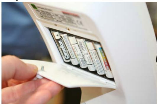
Figure 2-7. Batteries in Battery Chamber
