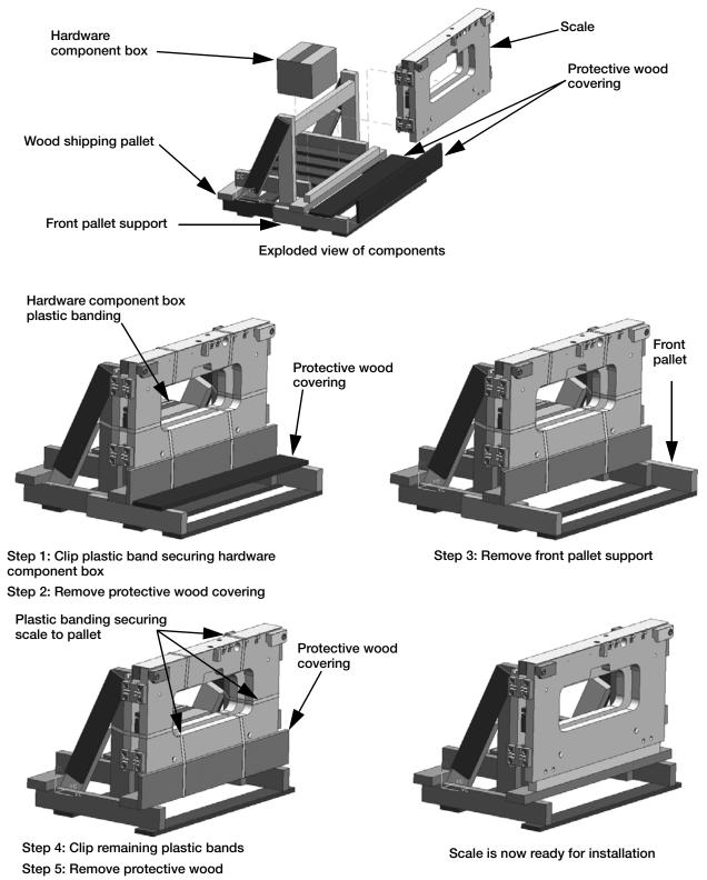
Figure 2-2. Scale Component Parts on Shipping Pallet for One Scale
