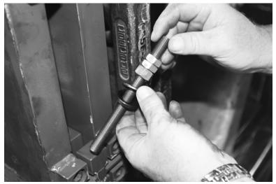
Figure 6-10. Install Spherical Washer Set
