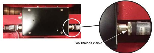
Figure 7-4. Connect Load Cell Cable to J-Box
