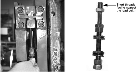
Figure 6-8. Installing Flexure into Scale
