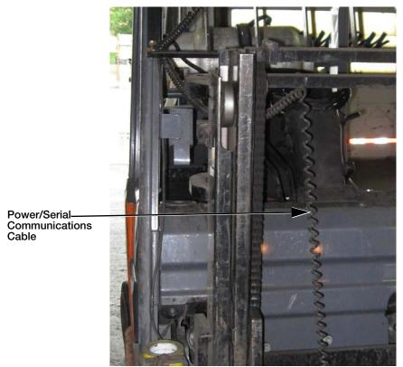
Figure 3-8. Signal Cable Located Between the Scale and the Indicator
