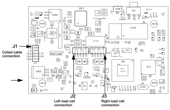
Figure 7-6. PCB Board Assembly
