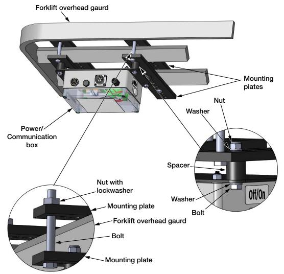
Figure 3-1. Power/Communication Box Installation
