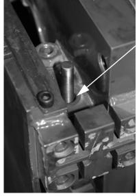
Insert the flat-blade screwdriver here to help center the flexure rod.
