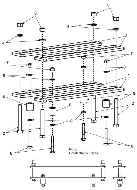
Figure 8-6. Plate Assembly, Power/Communication Box Cage Mount
