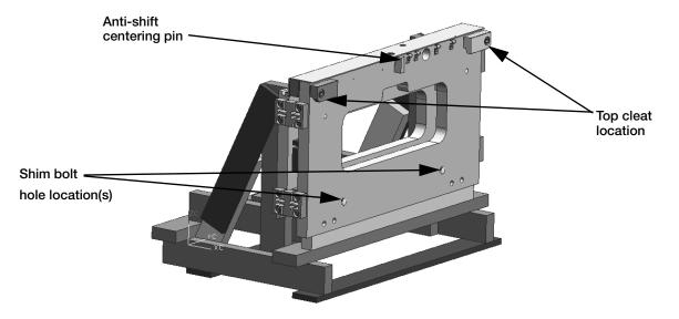
Figure 2-4. Anti-shift Centering Pin, Shim Bolts and Top Cleat Locations (One Scale Configuration Shown)
