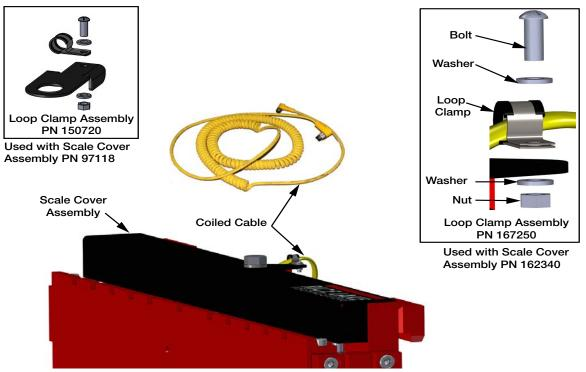
Figure 2-6. Connecting the Coiled Cable
