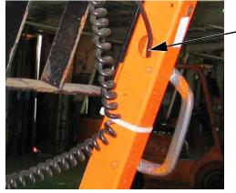
Run power cable through chassis to forklift battery.
