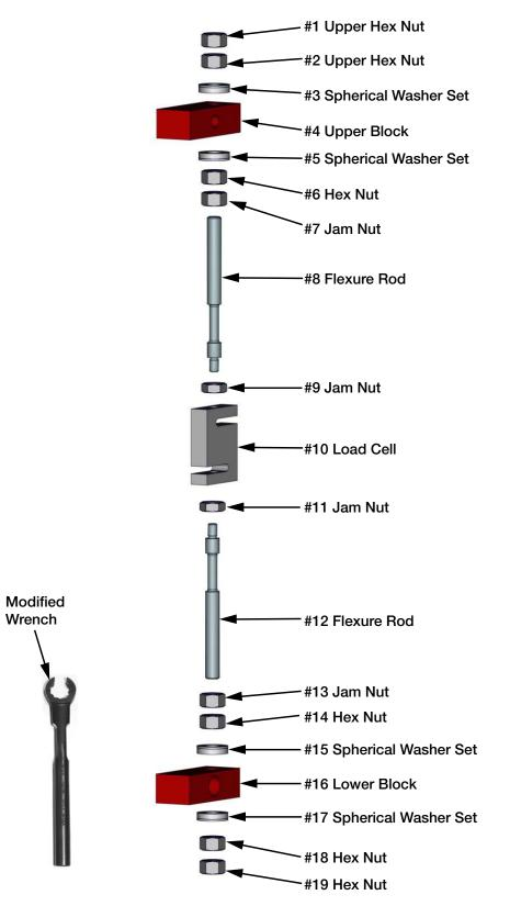
Figure 6-1. CLS-M Load Cell Assembly Parts Breakout
