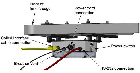
Figure 3-9. Power Switch on Power/Communication Box
