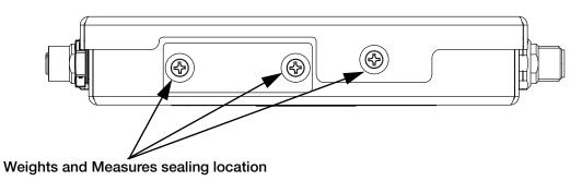
Figure 3-21. Sealing the J-Box for Weights and Measures
