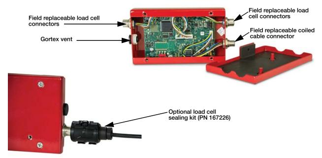
Figure 1-4. iQube2 Junction Box Component Parts
