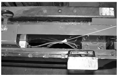
Detach load cell clip from back plate of scale using a large screwdriver.
