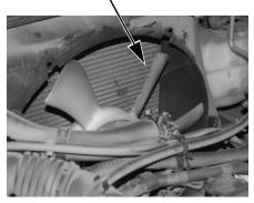
DO NOT route power cable close to objects that generate heat such as exhaust pipes.
