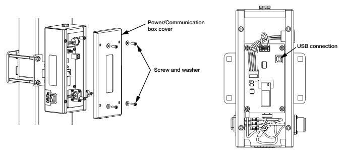
Figure 4-10. Connect USB to Power/Communication Box (PN 153616)
