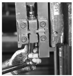
Figure 6-13. Tightening the Lower Hex Nut
