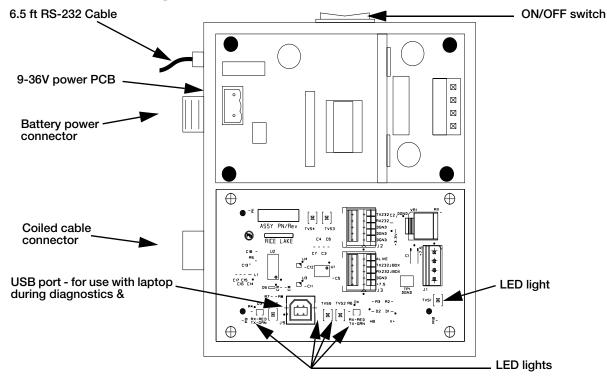
Figure 1-1. Power/Communication Box Schematic
