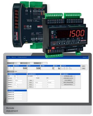
The integrated web server allows operators to remotely monitor, calibrate and configure the fieldbus models of SCT-4X, SCT-1SX and SCT-2200.
