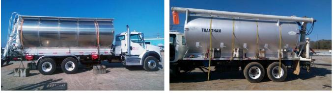
**CAUTION** DO NOT place straps or other load bearing supports on tanks without first ensuring that there is not a risk of damage to the tank structure.
