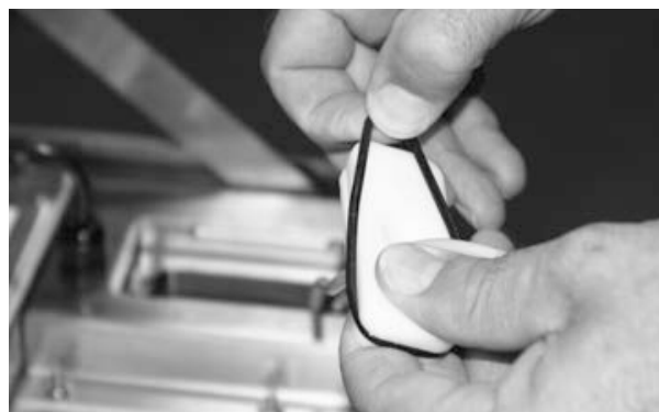
Figure 2-8. Assemble Split Seal Plates Together
