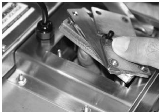
Figure 5-21. Remove the Component Parts of the Communications Cable Assembly
