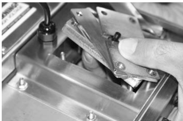
Figure 2-3. Remove the Component Parts of the Communications Cable Assembly
