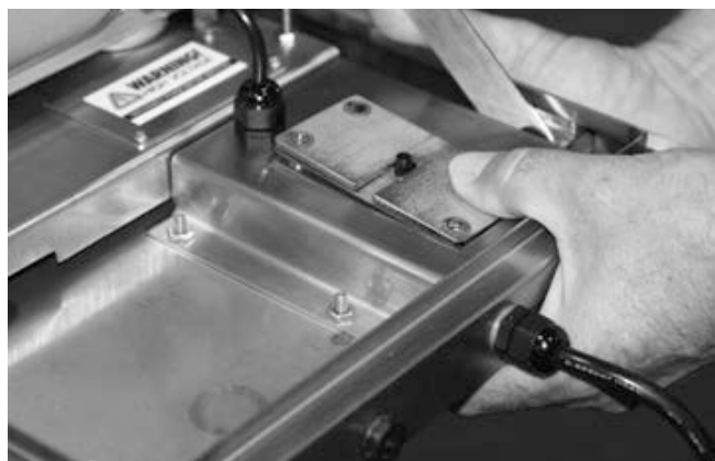
Figure 2-3. Remove the Component Parts of the Communications Cable Assembly
