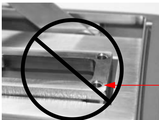
Figure 5-27. Incorrect and Correct Orientation of Main Plate
