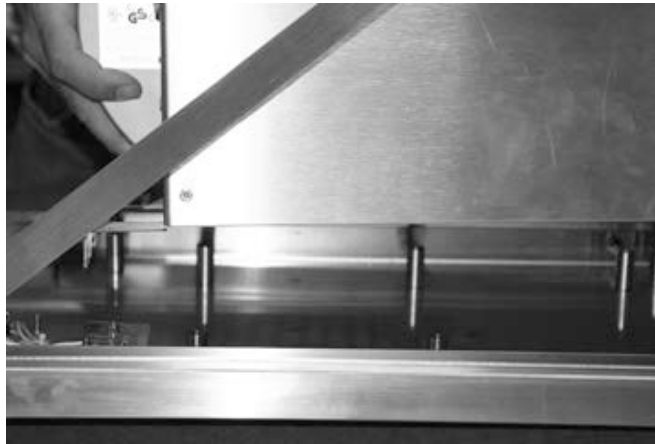
Figure 5-6. Pull Printer and Mounting Pad Off Base Plate
