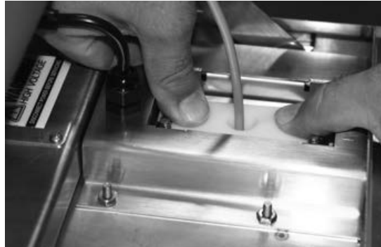
Figure 5-29. Seat the Split Seal Assembly
