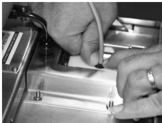
Figure 2-11. Insert Split Grommet Onto the Split Seal Plates
