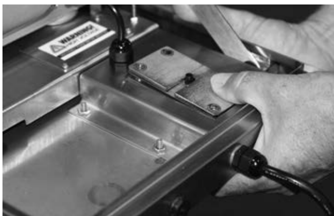
Figure 5-21. Remove the Component Parts of the Communications Cable Assembly
