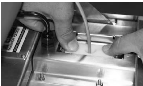
Figure 2-10. Seat the Split Seal Assembly
