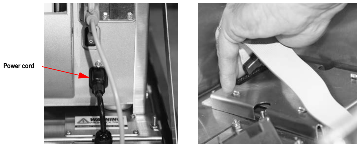
Figure 5-4. Disconnect Power and Printer Cables
