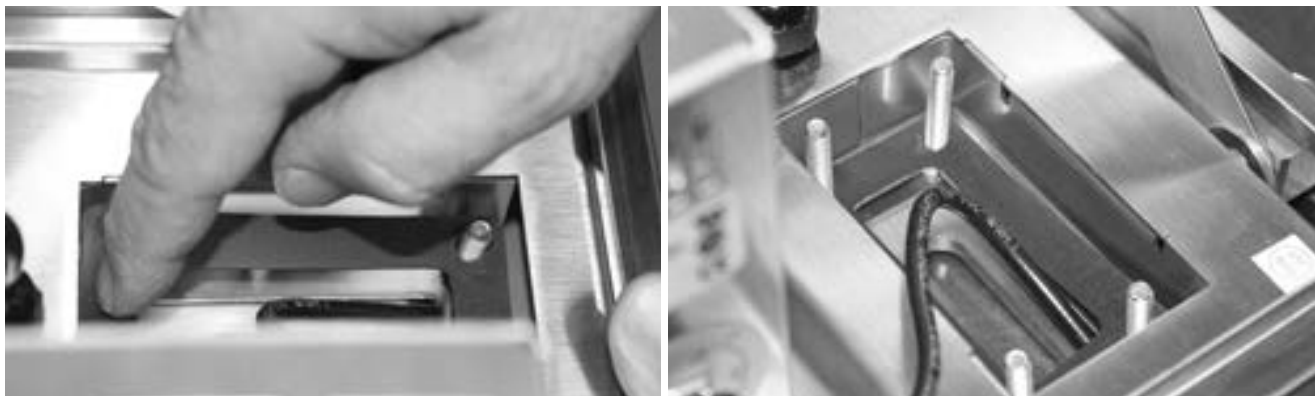
Figure 5-26. Press Down Rubber Gasket Around Bolts
