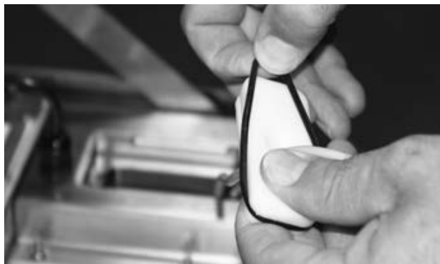
Figure 5-28. Assemble The Split Seal Plates Together
