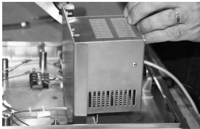
Figure 5-10. Secure Heater to Enclosure Bottom
