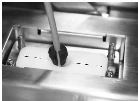
Figure 2-11. Insert Split Grommet Onto the Split Seal Plates
