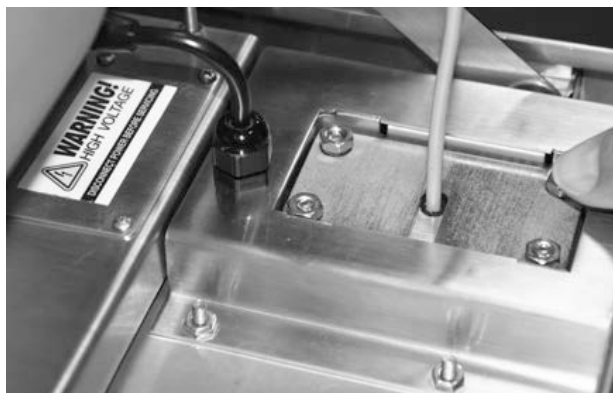
Figure 2-13. Tighten Up The Entire Assembly
