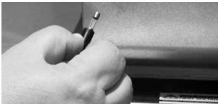
Figure 5-19. Remove Actual Fuse From the Receptacle and Replace with a New Fuse
