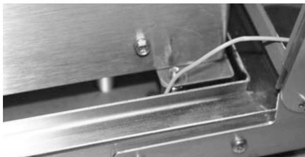
Figure 5-15. Don't Pinch Ground Wire
