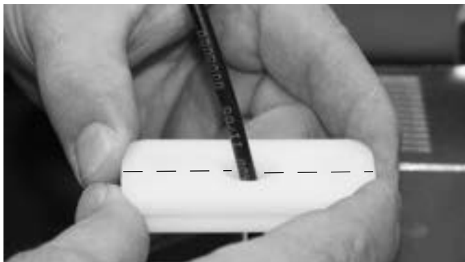
Figure 5-28. Assemble The Split Seal Plates Together
