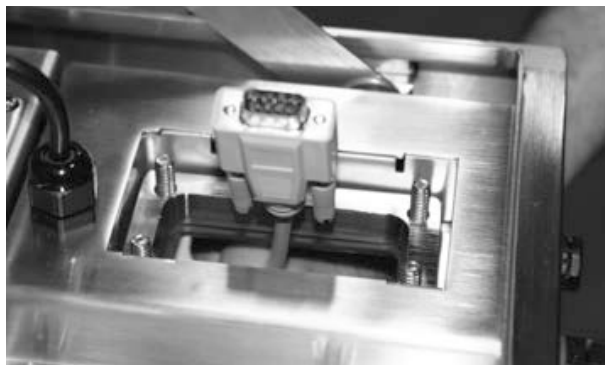
Figure 2-7. Communications Cable Comes Up Through Bottom of Hole
