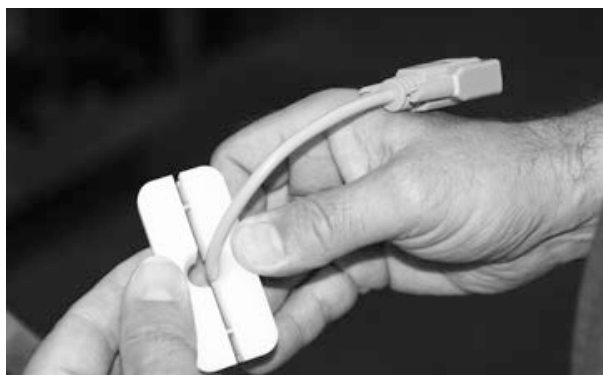
Figure 2-8. Assemble Split Seal Plates Together
