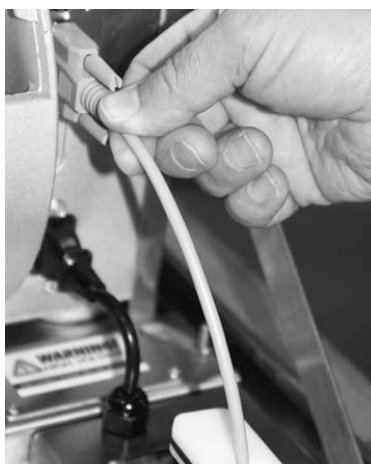
Figure 2-9. Connect Communications Cable to Back of Printer
