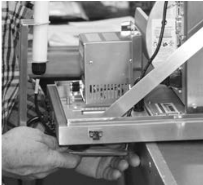
Figure 5-25. Installing Antenna Kit Bolts and Cable Through Printer Base
