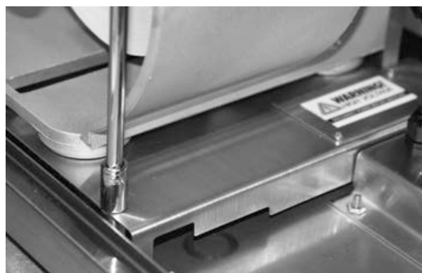
Figure 5-16. Secure All Four Nuts Holding Printer Pad to Enclosure Bottom
