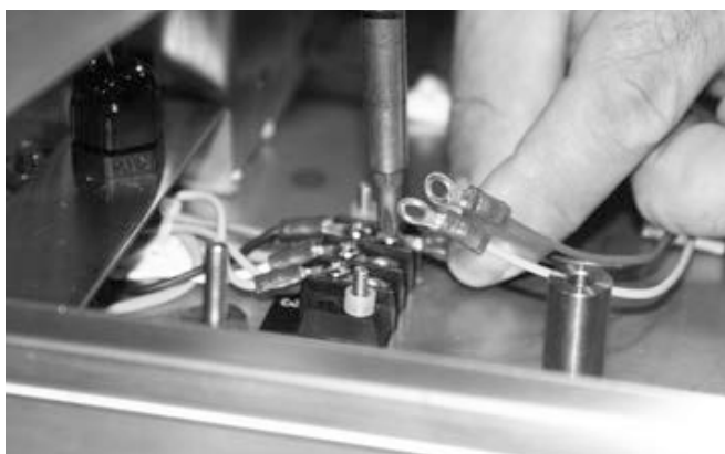
Figure 5-11. Color Match Wire Harness and Terminal Strip Wires
