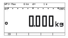
Press (ISO-Test) to start an external adjustment.
