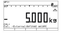
➤ You are prompted to place the required weight on the platform (e.g.: 5.0 kg). The subsequent steps for completing the calibration/adjustment are described in the chapter entitled "Operation" under "Calibration and Adjustment."
