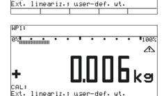
After a short time the difference between the measured value and the true weight of the sample will be displayed.
