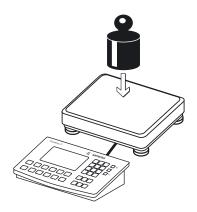
▶ Place the calibration/adjustment weight on the weighing platform.
