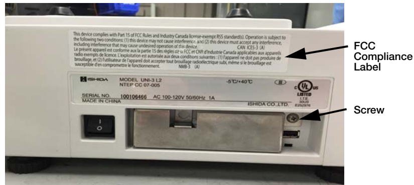
Figure 6. Secure Cover with Screw and Apply FCC Compliance Label
