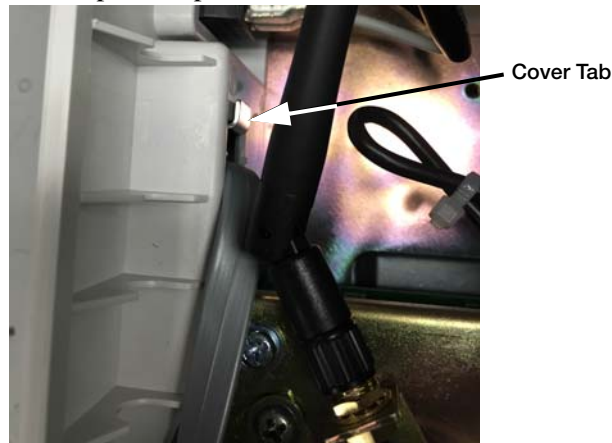
Figure 5. Insert Stainless Steel Cover
