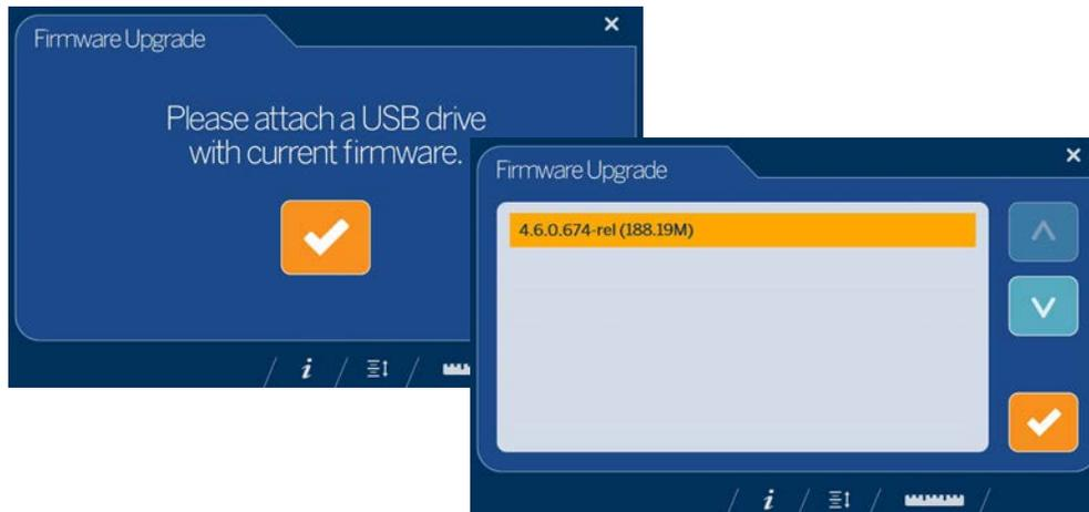
Figure 4-9. Connect USB Drive to Upgrade Firmware
