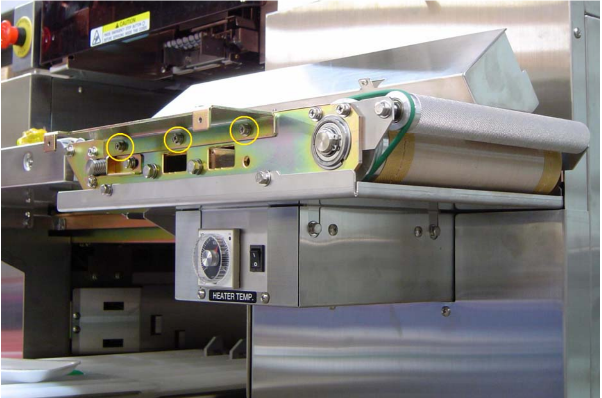
Figure 3. Heater Conveyor front frame.
