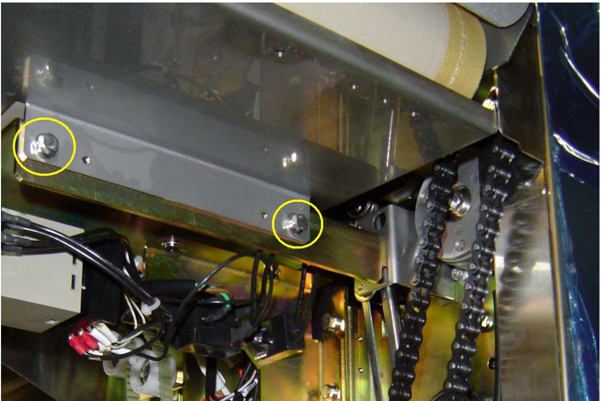
Figure 7. Heater Conveyor mounting bolts (two of four).
