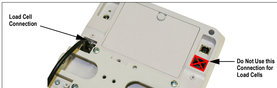
Figure 2-10. Load Cell Connection Point
