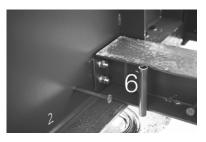
**Number 7 cross beams** make up the rest of the beams in the middle area of each module. Short modules may have only one or two #7 cross beams, while longer modules may have four or more. The #7 beams are similar to #6 beams, but don't have the extra 3/8" threaded studs near their ends. Any #7 beam can be reversed end-for-end so drain tubes can be staggered from side to side for even drainage from the deck.
