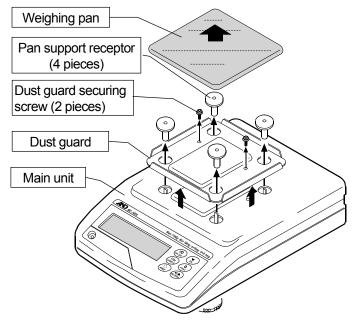
Secure the breeze break to the main unit using two screws provided with the breeze break.
