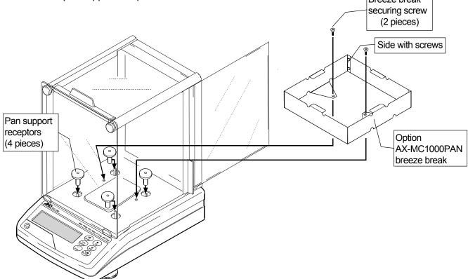
2. Place the auto-centering pan guide on the pan support receptors, and then place the auto-centering pan on the guide.
