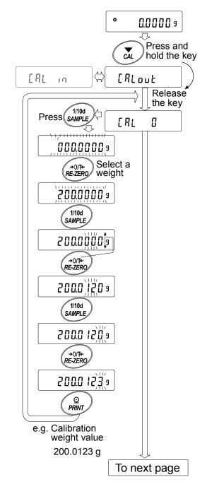
5 Confirm that there is nothing on the pan and press the PRINT key. The balance measures the zero point. Do not allow vibration or drafts to affect the balance.
