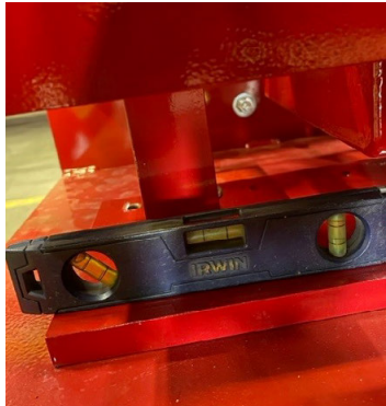
Figure 4-8. Recheck Link for Binding
