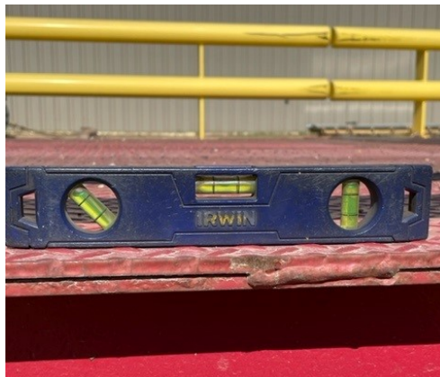
Figure 3-8. Check Weighbridge for Level
