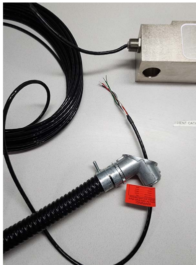
Figure 4-2. Insert Load Cell Cable Through 90° Fitting
