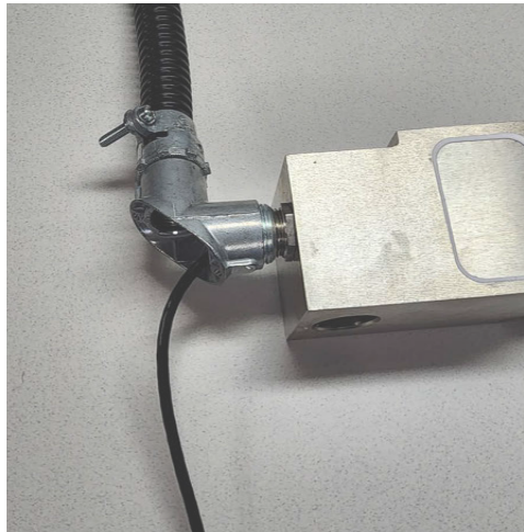
Figure 4-3. Installing 90° Fitting to Load Cell
