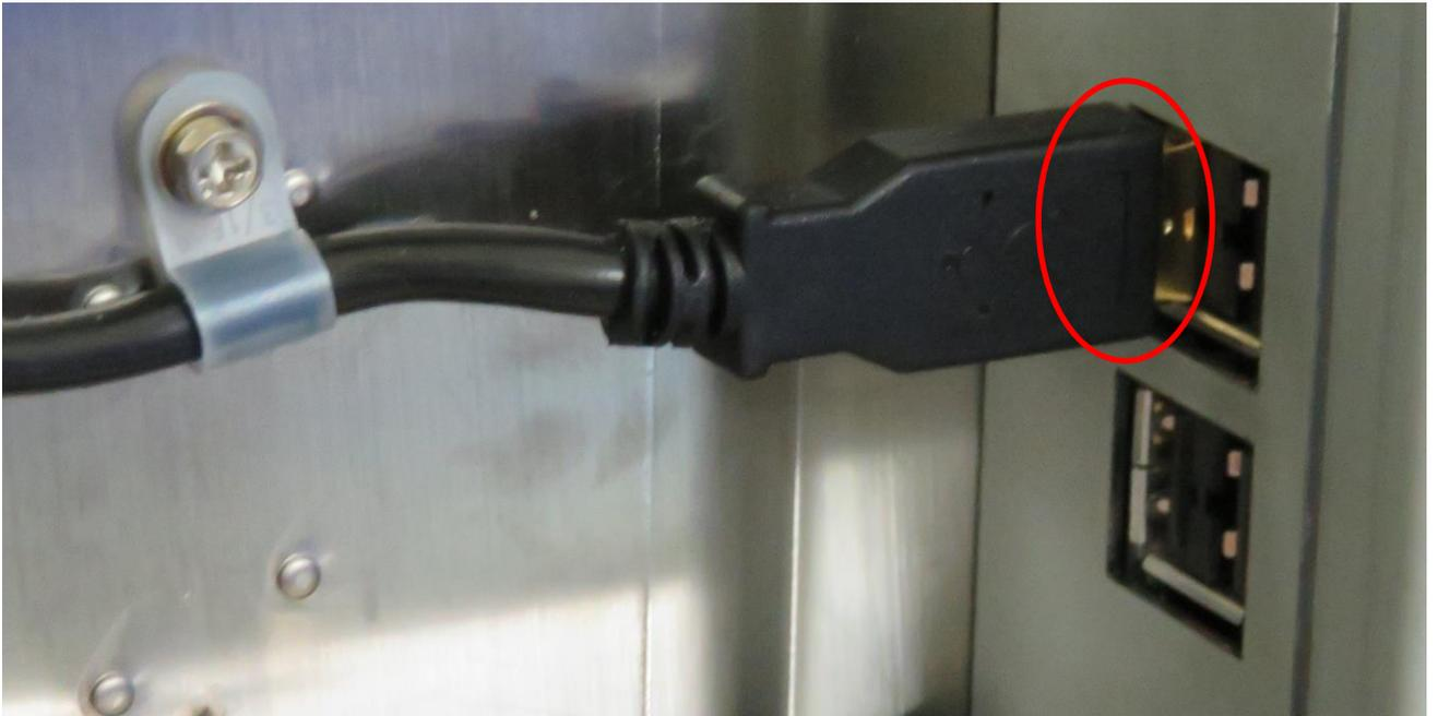
The line from P-1100\* A10 to P-1131\*-3 A410. Refer to the picture for USB plug connecting position.
