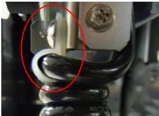
6. To confirm that there is no tensioning or passing each other of the curled code to move the suction block by hand.
