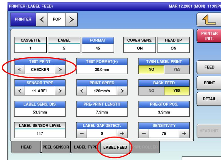
Label sensor distance: Select [CHECKER] for [TEST PRINT], measure the position of a ruled line of thermal print, which is located above an address / store name, from the bottom of the label. Enter a value in [LABEL SENS. DIS.] shown on the screen below so that the measured size and the value inputted in [PRE-PRINT LENGTH] become the same.
