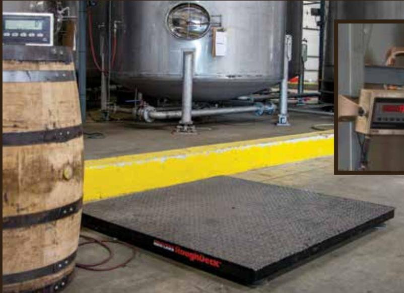
*RoughDeck floor scales weigh barrels and totes while 320IS indicators display weights at various stages of bourbon production. Intrinsically-safe equipment is installed throughout the distillery.*
