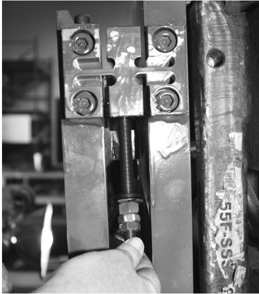
Figure 6-78. Installing Flexure into Scale
