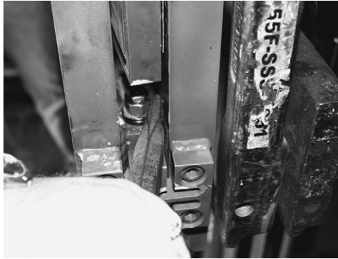
Figure 6-82. Centering the Load Cell Using a Chisel
