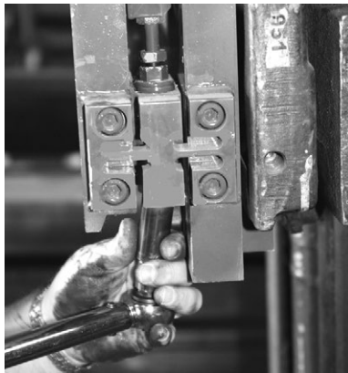
Figure 6-83. Tightening the Lower Hex Nut
