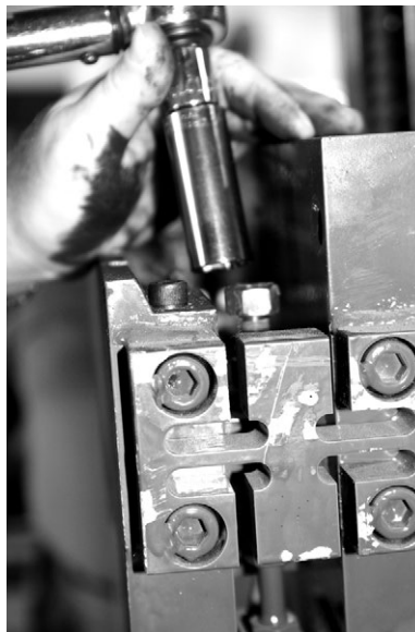
Figure 6-72. Removal of Hex Nut (#1 of Parts Breakdown)
