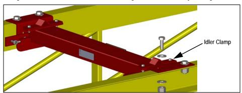
Figure 2-9. Installed 711 Weighframe
