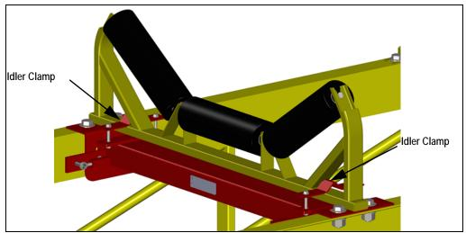
Figure 2-10. Install Idler on 711 Weighframe
