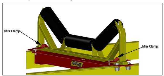
Figure 2-4. Install Idler On Weighframe
