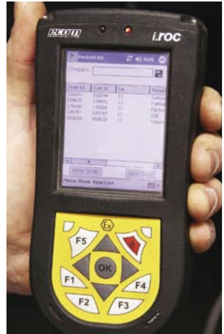
CRS is installed on an explosion proof PDA for intrinsically safe environments.
