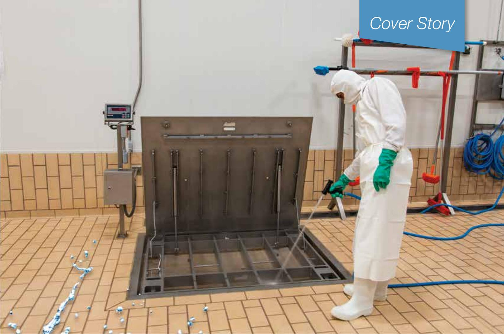
*The QC-X floor scale's top plate opens to 75 degrees for unmatched cleaning access. They are routinely blasted with high-pressure hot water to remove any post-weighment food residue.*
