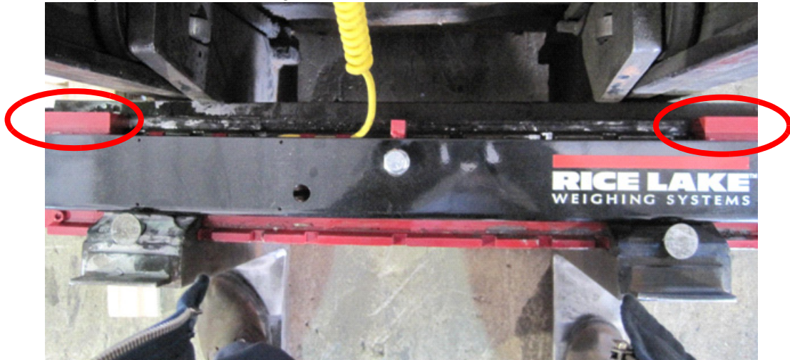
Figure 5. Top View of Rice Lake Weighing Scale Installed
