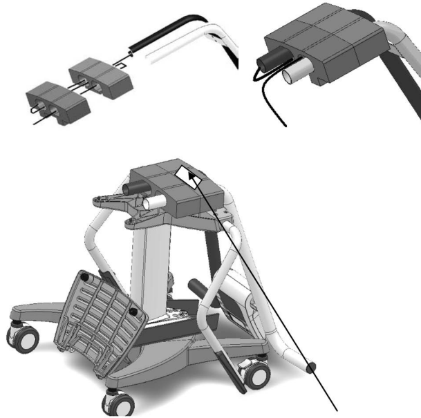
Figure 2-7. Remove Styrofoam Packing Pieces From Main Handle
