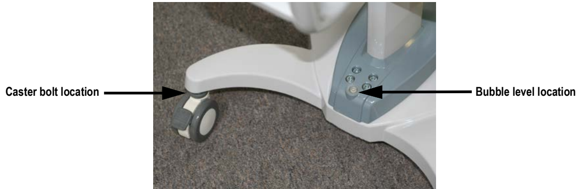
Figure 2-14. Bubble Indicates That The Scale is Level
